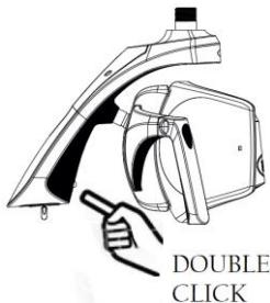
Each time a double click is performed, the Tk of the light changes. Repeat the procedure until the desired colour temperature is displayed on the indicator light. 2 beeps will inform the user that the Tk is changing.
