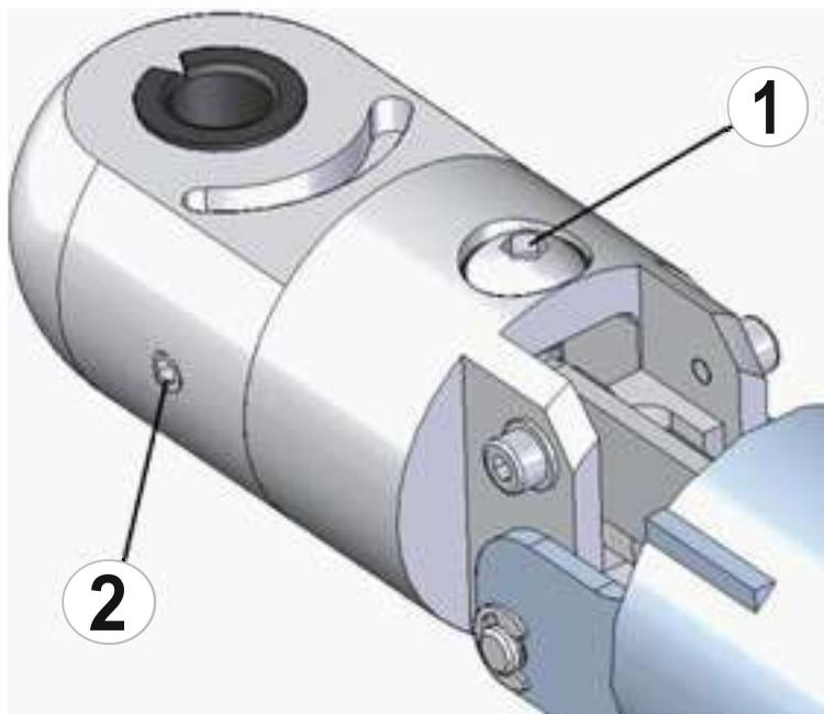
With the adjusting screw, the tray can be aligned in its radially horizontal position.
